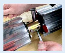
**EASY CONNECTOR INSTALLATION** Three flexible connectors between the rollers allow Lake Groomer to follow the contour of the lake bottom. Just one bolt is required to attach or detach the rollers, so changing your roller configuration is simple!
