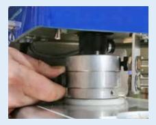
ADJUSTABLE ROLLER ARC The roller path can cover an arc up to 280 degrees and is easily adjusted with the directional pucks. When they reach the end of their set arc, the rollers will automatically reverse and continue rolling.
